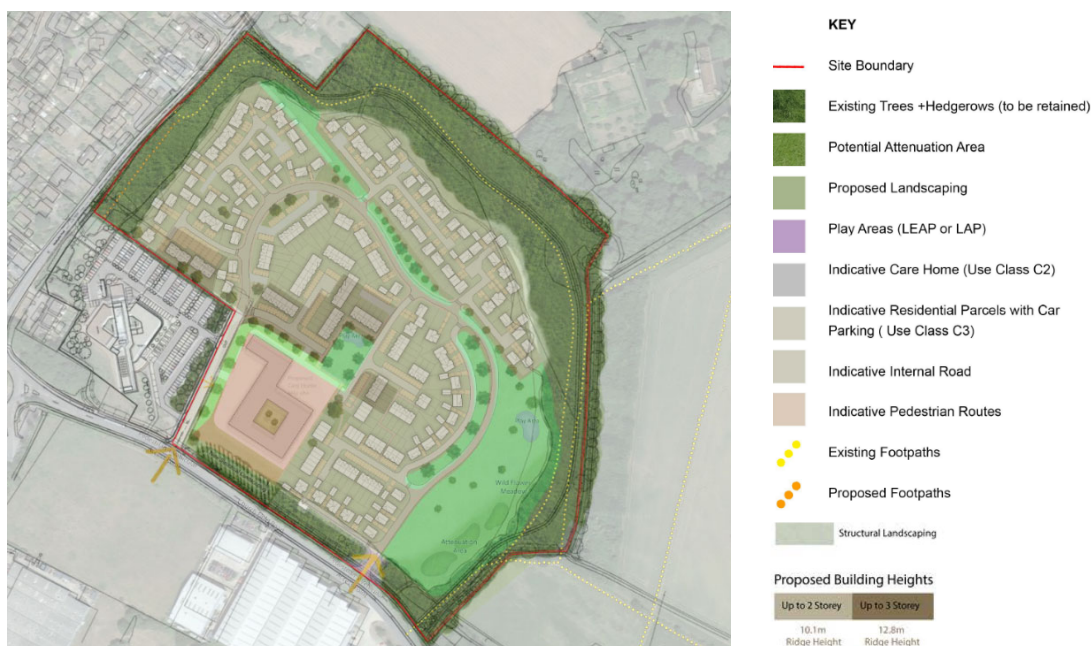
Figure 3: KLH Parameters Drawing overlaid with the Indicative Masterplan to show the height an extent of development, encroaching 18.5m into the G3/G7 plantation along the northern boundary with Chilton Hall.
